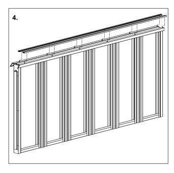
4. Mount the aluminium dust sealing profiles on the run-through jamb. Use a wooden or rubber hammer for this.
