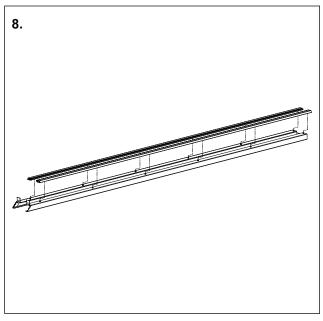
8. Mount the aluminium dust sealing profiles on the closing jamb. Use a wooden or rubber hammer for this.
