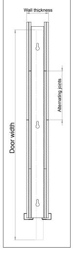
19. The closet part is now ready to be finished with 12,5 mm plasterboard
