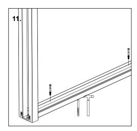
11. Install the ground ruler of the niche closet. PAY ATTENTION, the ground ruler should be parallel with the two lines and exactly in the middle.
