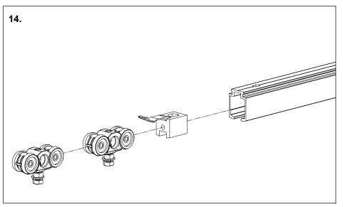
14. **PAY ATTENTION:** if not softclose, place the trolleys, and if fixation of the door is desired, place the end stopper in the rail.
