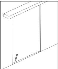
8. Check the floor beforehand using a long level for angularity and flatness. You can take this information into account during the placement of the element.
