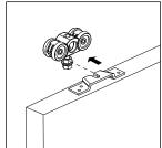
16. Hang the door with the bearing plates on the trolleys. First the backside, then the front.
