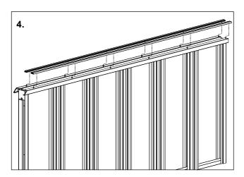
4. Mount the aluminium dust sealing profiles on the run-through jamb. Use a wooden or rubber hammer for this.
