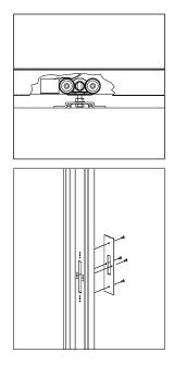
18. Push the door buffers in the holes of the closing jamb.
