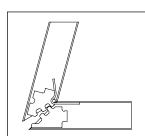
10. Place the closing jamb with a turning motion around the wall such that the miters grip correctly into each other.
