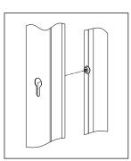
7. Place the aluminium rail in such a way that the pre-assembled brass fasteners fit into the keyholes of the niche closet and allow the rail to slide in place.
