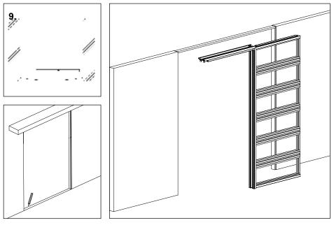
9. Check the floor beforehand using a long level for angularity and flatness. You can take this information into account during the placement of the element.
