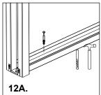
12. Install the ground ruler of the niche closet. PAY ATTENTION, the ground ruler should be parallel with the two lines and exactly in the middle.
