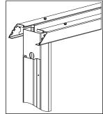
3. Place the niche closet with the open side upwards on the floor. Mount the run-through jambs using the parker head screws.
