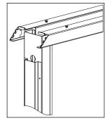
3. Place the niche closet with the open side upwards on the floor. Mount the run-through jambs using the parker head screws.
