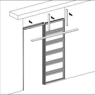
13. Connect the end profile of the niche closet to the wall and fill the space between closing jamb and wall with multiplex.
