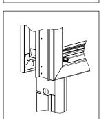
6. Place the transom of the frame by means of a turning movement in a horizontal position in relation to the niche closet.
