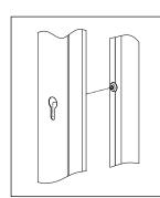
6. Place the aluminium rail in such a way that the pre-assembled brass fasteners fit into the keyholes of the niche closet and allow the rail to slide in place.
